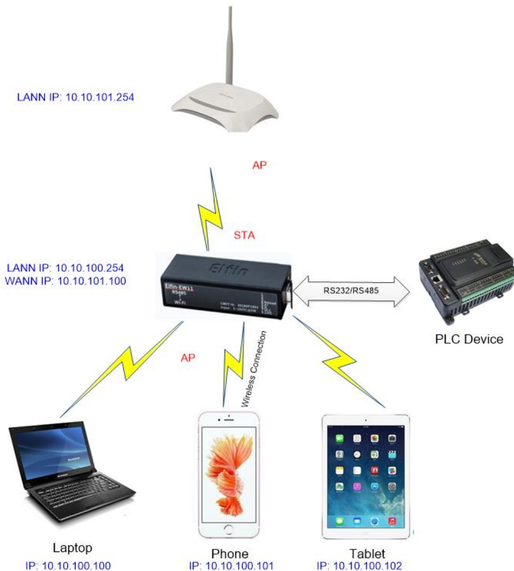
Figure 24. AP+STA Wireless Network
