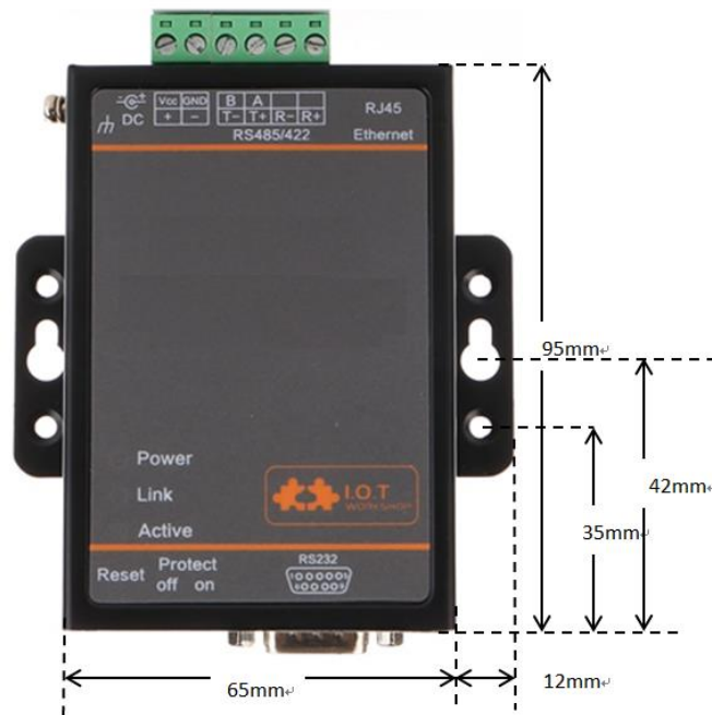
Figure 7. HF2211 Mechanical Dimension
