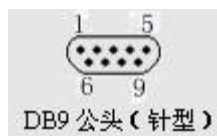
Figure 4. RS232 Pin Defination(Male/Needle Type)
