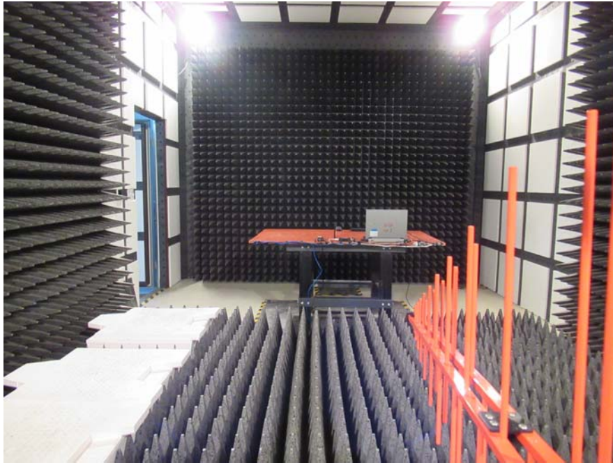
RS Test Setup photo
