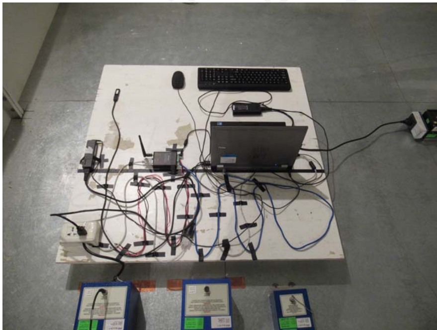
CS Signal Port Test Setup photo
