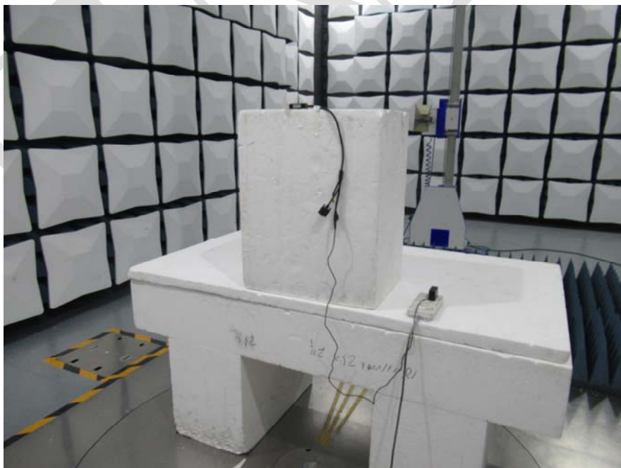
Radiated Spurious Emissions Test View (Above 1GHz)
